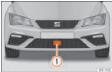
Fig. 266 On the front bumper: radar sensor.
