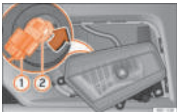
Fig. 114 Fog light: detach the bulb holder
