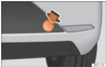
Fig. 102 Right side of the rear bumper: cover-cap.
