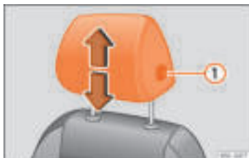
Fig. 20 Front seat: adjusting the head restraint.
