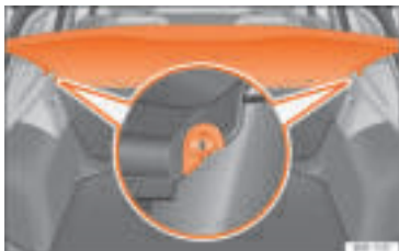
Fig. 172 In the boot: removing and installing the shelf.
