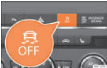
Fig. 257 Centre console: Button for switching on/off the ESC and ASR
