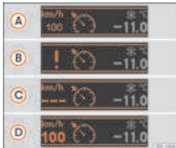
Fig. 264 Instrument panel display: CCS status indications.
