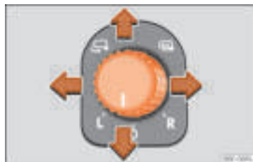
Fig. 158 Driver door: control for the exterior mirror.
