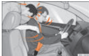
Fig. 95 The unbelted passenger in the rear seat is thrown forward violently, hitting the driver who is wearing a seat belt.
