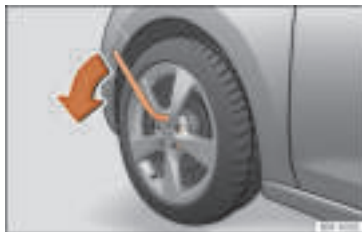
Fig. 77 Wheel: loosen the wheel bolts.
