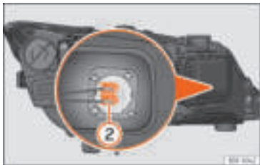
Fig. 112 Main beam headlight bulb.
