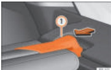
Fig. 174 In the luggage compartment: remove the shelf.
