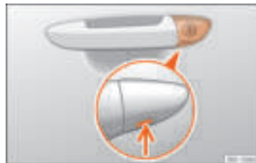
Fig. 6 Driver door lever: hidden lock cylinder.
