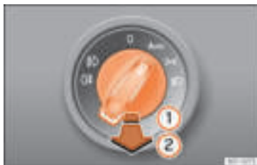
Fig. 151 Instrument console: light panel.
