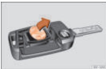
Fig. 146 Vehicle key: removing the battery.
