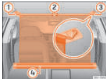
Fig. 182 In the boot: net partition hooked into the rear seat backrests. »
