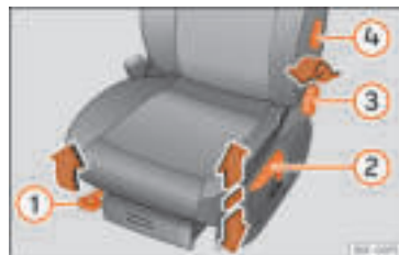
Fig. 18 Front seats: manual seat adjustment.
