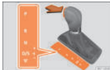
Fig. 56 Automatic transmission: selector lever positions.
