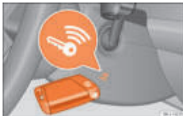
Fig. 253 On the right of the steering column: emergency start.
