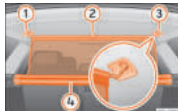
Fig. 179 In the boot: securing the partition net.
