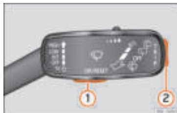
Fig. 136 Windscreen wipers lever: control buttons.
