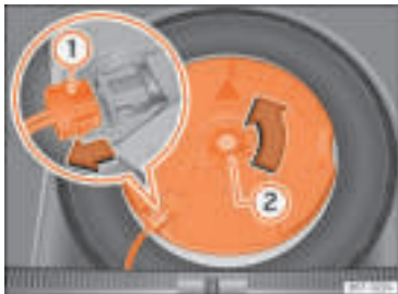
Fig. 318 In the boot: remove the subwoofer.
