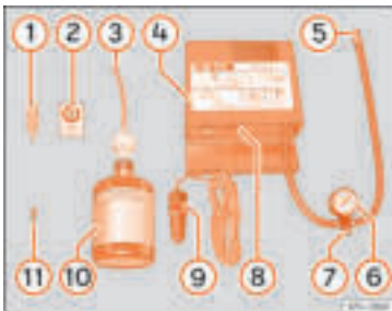
Fig. 71 Standard display: contents of the anti-puncture kit.
