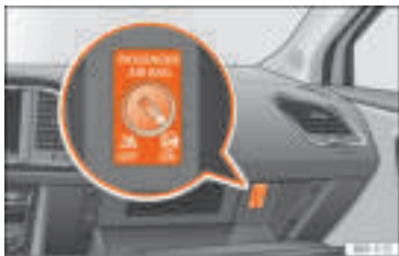
Fig. 28 Front passenger front airbag switch.
