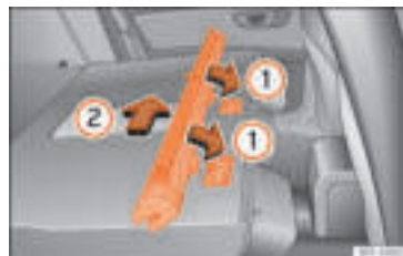
Fig. 181 Assembling the net partition in the rear seat backrests.
