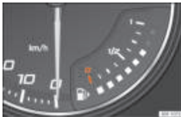
Fig. 131 Analogue instrument panel: fuel gauge
