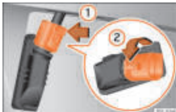
Fig. 122 Number plate light: detach the bulb holder.
