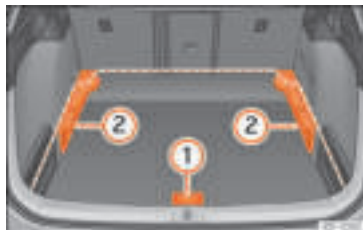
Fig. 193 Variable boot floor: position.
