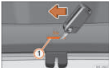
Fig. 9 Luggage compartment: access to manual release.
