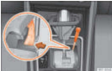
Fig. 57 Selector lever: manual release from position P.
