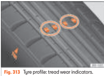
Fig. 313 Tyre profile: tread wear indicators.
