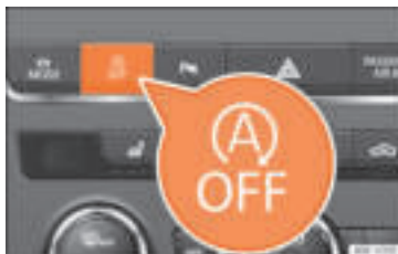
Fig. 262 Centre console: Start-Stop system button.
